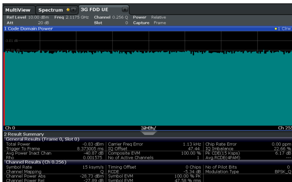
Fig. 9-5: Measurement Example 3: Measuring the Relative Code Domain Power with Incorrect Scrambling Code
