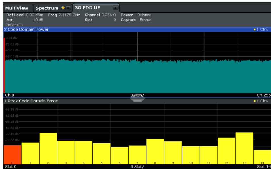
Fig. 9-8: Measurement Example 6: Determining the Peak Code Domain Error
