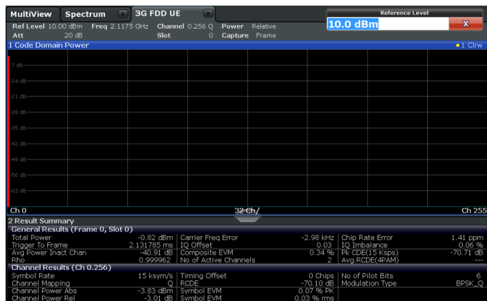
Fig. 9-3: Measurement Example 3: Measuring the Relative Code Domain Power
